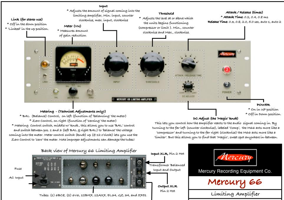
**Link Input**, This lets you 'link' two (2) Mercury 66 Limiting amplifiers together for Stereo applications.
